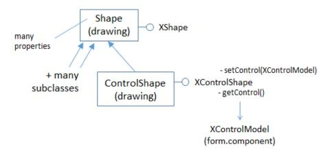
Figure 2. The Shape and ControlShape Services.
